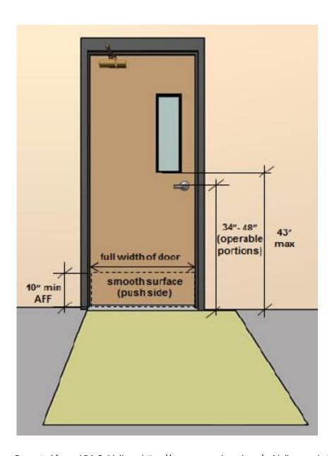
Vision/ Side Lights (if provided) (§404.2.11) Accessible viewing height 43" max. unless not intended for viewing (i.e., lowest part above 66")
